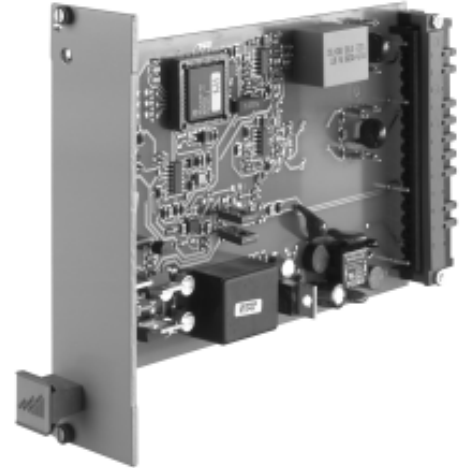
Fig. 1. EURAX F 534 as plug-in module for 19" rack-mounted case, front plate width 7 TE.
